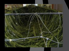
Hull construction – Having done first steps in vacuum infusion four years ago, going to the next level of vacuum infusion with cutting edge VAP membranes (the process that are used in building production of Airbuses) was natural development in our boat building process. Application of clear gelcoat under the water line for added strength and full checkout is performed as well.
